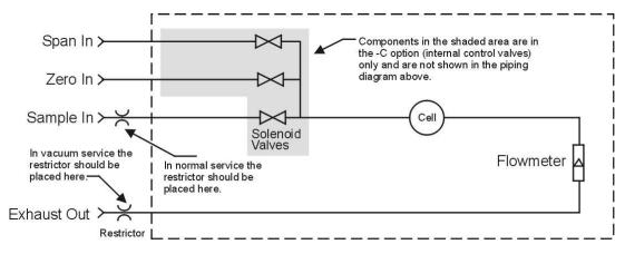
Figure 2-2: Flow Diagram with Options
